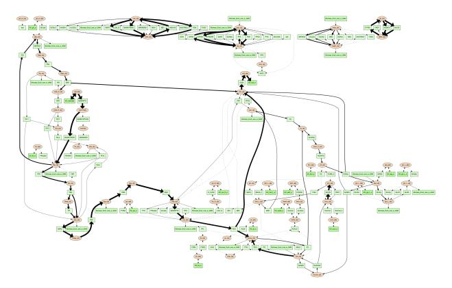
Reactions with a flux of zero is represented as a dotted edge and non-zero fluxes as solid. Meanwhile, the thickness of the edges is proportional to the flux through the reaction. Visualizing these fluxes may help highlight reactions that contribute the most to the objective.
